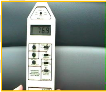
The sound test was conducted using the Cirrus Sound Meter (above)
