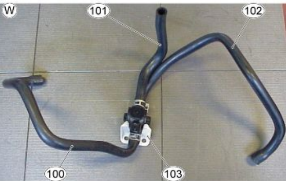
CENTRAL W - FITTING THE PIPES ON THE SECONDARY AIR SOLENOID
