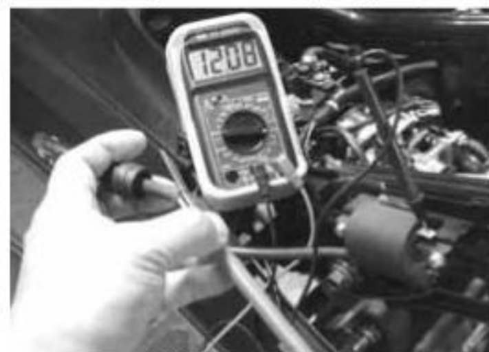
Secondary Coil without plug cap
